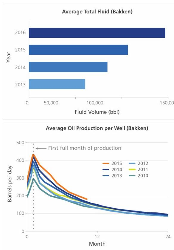
Figure 1: Yearly average total fluid volumes and production curves in the US Bakken. (Sources: NavPort Analytics, U.S. EIA)
