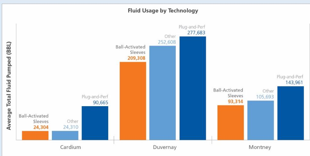
Figure 4: Comparison of average fluid volumes pumped for completions in major formations in Canada. (Source: geoLOGIC Systems)
