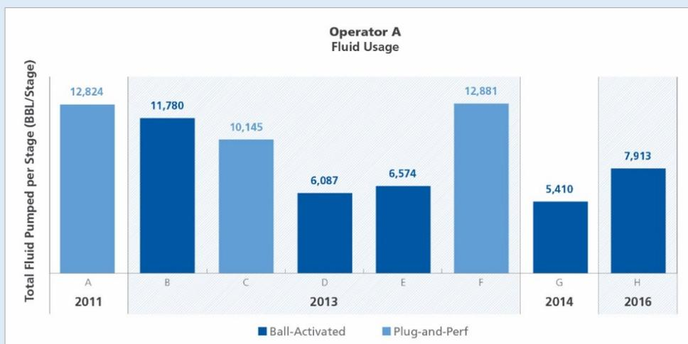
Figure 3: Comparison of fluid usage for ball-activated versus plug-and-perf completions in the Montney. (Source: geoLOGIC Systems)
