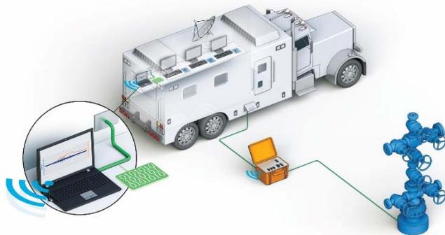
Connectivity between the wellhead, Retina data acquisition box, data van, and Retina laptop.
