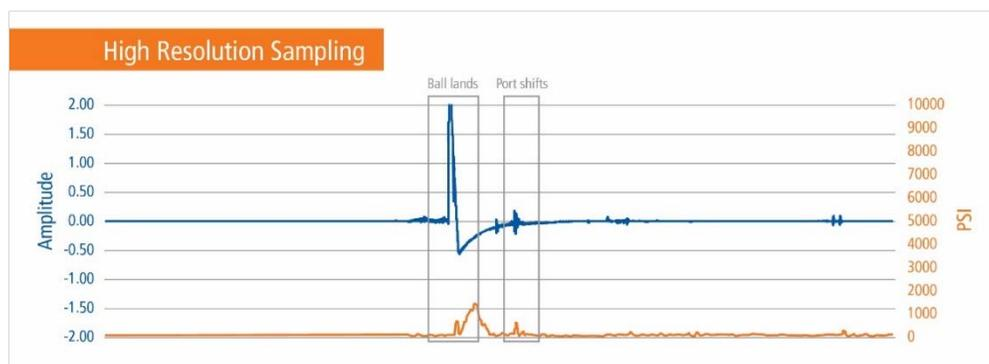
Retina shows the ball landing on seat and shifting, both within 0.4 seconds. The pressure signature was not seen in the data van.
