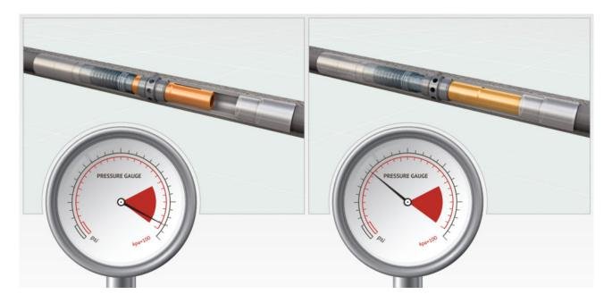
The Toe-XT Testable Hydraulic Sleeve is specially designed to operate with a dual pressure cycle that enables a high pressure casing integrity test (pictured at left) and a low pressure sleeve opening that is independent of stimulation operations (pictured at right).
