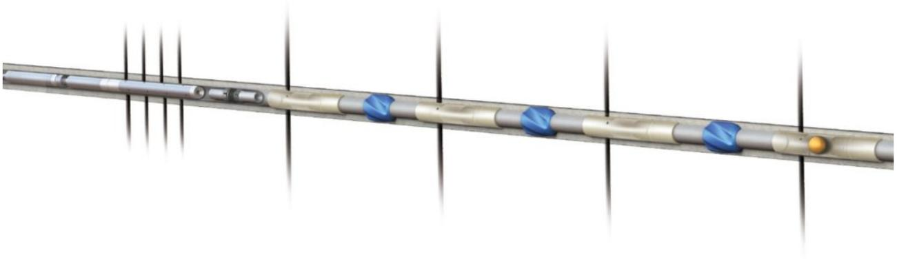
TREX limited entry hybrid completion solution consisting of QuickPORT IV sleeves at the toe followed by plug-and-perf stages
